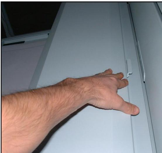
Close the covering of the stacker by pressing it downwards in the middle until it snaps in on both sides.
