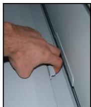
In case of a paper jam the stacker covering can be tilted upwards and the distracting paper can be removed.
